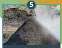
Heated gully waste material leaving the drying process.
