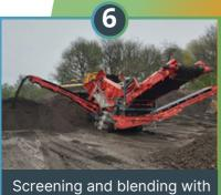
Screening and blending with soil and nutrients to produce 10mm topsoil.
