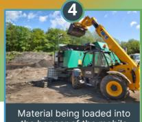
Material being loaded into the hopper of the mobile mineral drier.
